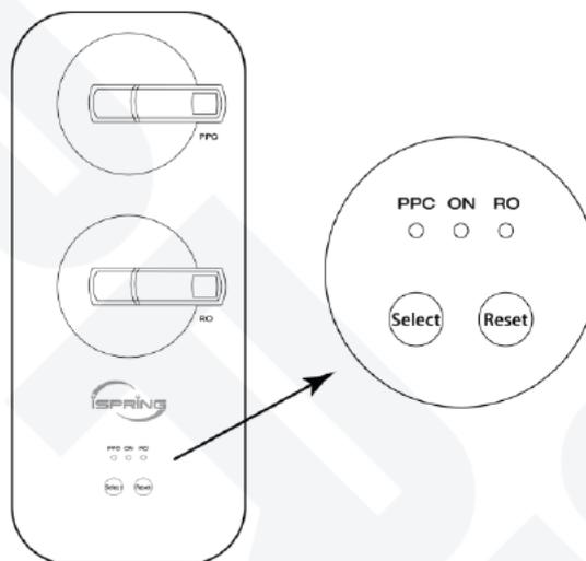
The display/Operating area is located in the lower front side of the system that is made with a combination of 3 indicating lights and 2 buttons.
