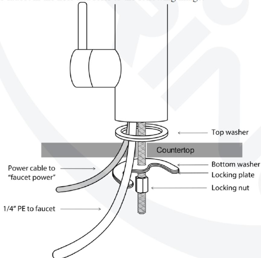
▪ **Connect the System with Power Cable and PE Water Tubing**
