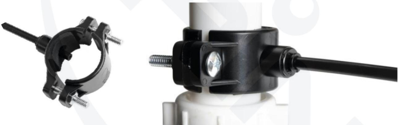
**Step 3. a.** Choose a proper spot anywhere before the P-trap on the drain pipe to install the drain saddle and tubing. Remember the drain saddle should NOT be installed after the P-trap to prevent potential microorganism growth.
