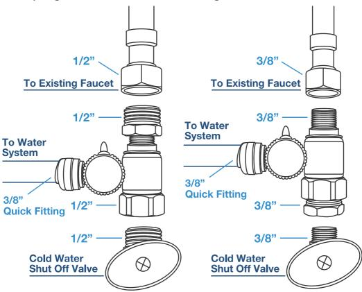
The included Conversion Adapter (bushing) can be threaded on either side of the valve to make a configuration of 3/8" x 3/8" COMP or 1/2" x 1/2" NPT.
