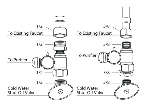
The included bushing can be threaded on either side of the AFW38 to fit the 3/8" COMP and 1/2" NPT configuration.
