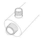
**Step8–** Hand-screw open end nut on the filter chamber (open-end of quartz tube). To protect the O-ring, do not overtighten.
