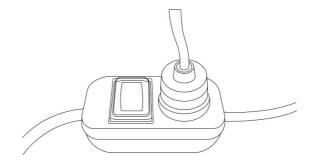
**Step 14–** Push control switch to the button "AUTO," the UV lamp will start working automatically when there only water flowing. Push control switch to button "MOVE," the UV lamp keep working continuedly. Push the control switch button "STOP" to turn off the UV lamp. Mode AUTO is highly recommended to protect the UV lamp.
