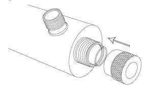
**Step 9**– Connect 4-pin electrical socket with UV lamp pins tightly.
