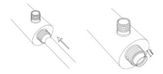
**Step7–** Hand-screw closed-end nut on the filter chamber(closed end of quartz tube). To protect the O-ring, do not overtighten.
