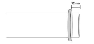
**Step5–** Insert the quartz tube into the filter chamber.
