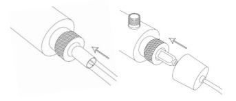
**Step 11–** Install the cover cap and hand-tighten it onto open End Nut.
