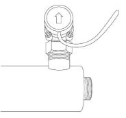
Step 13– Connect flow switch cable with control switch, close the switch cover.
