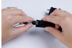
2) Plug the other end of the green wires into the big power socket of the lamp holder
