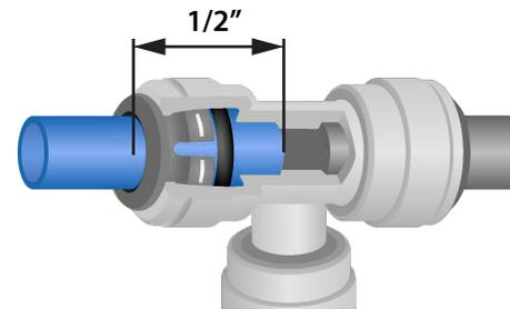
\*To connect, insert the tubing 1/2 inch deep until it's sealed by o-ring and locked by spider teeth.
