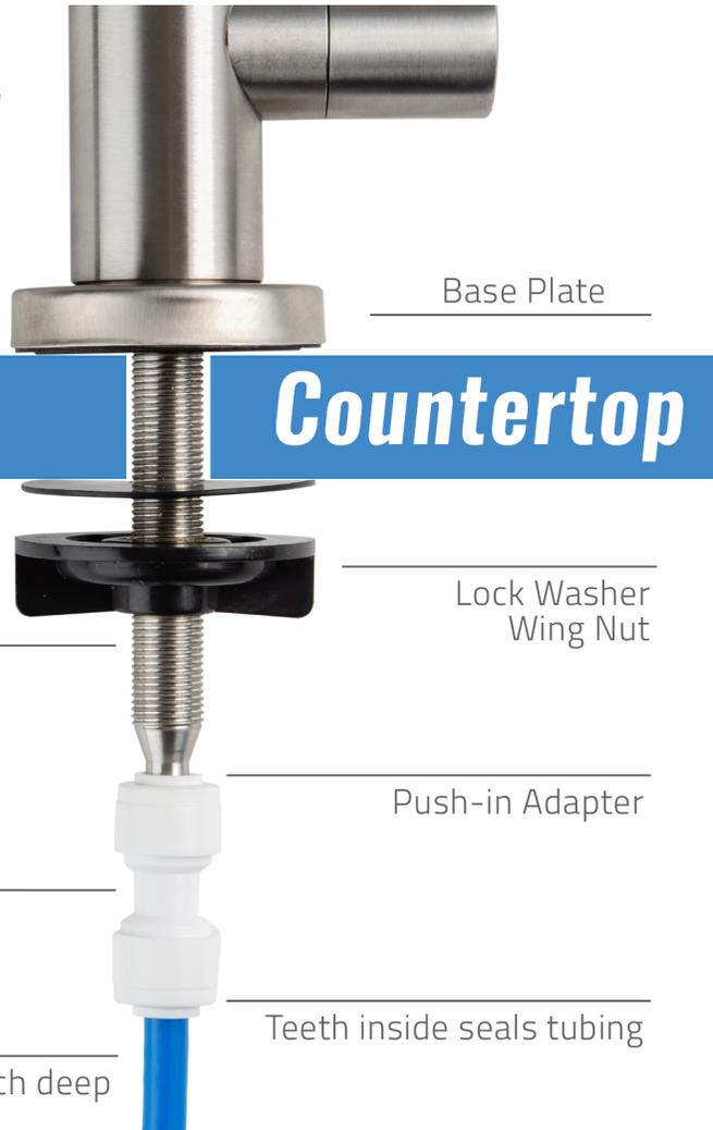
2. Slide the base plate onto the faucet stem. Insert the faucet stem into the hole on the countertop. Under the sink, insert rubber washer and tighten the wing nut (you may apply a few rounds of Teflon tape to the threads to get a better grip).
