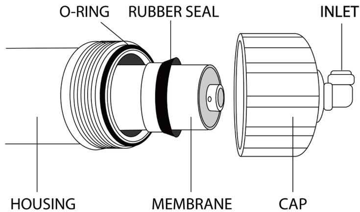
Place the membrane housing cap back, make sure the o-rings are in place on the housing, and hand tighten it. Use the housing wrench to tighten another ¼ - ½ of a turn.
