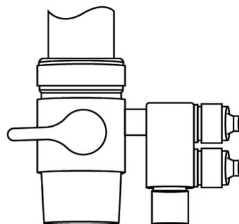
Check if there’s any leak inside the system or from the feed water valve. If there’s leak on the valve, make sure enough plumber’s tape has been applied and the adapter is tight enough. If there’s any internal leak, contact iSpring customer service immediately.
